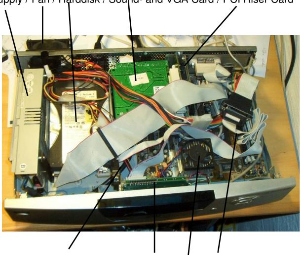
IRDA Receiver / LCD Display / CPU / Mainboard
